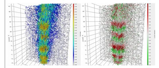
Figure 1. Shake-the-Box results for a free jet in water\*\*: velocity (left) and acceleration (right). Recorded, calculated and displayed in LaVision's *DaVis* software
